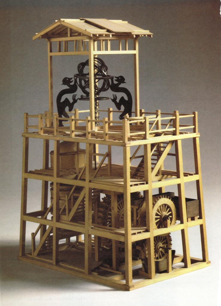
The first mechanical clock used a water wheel to create sounds every quarter hour.
